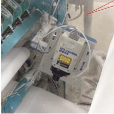
Accurate, non-contact length and speed measurement with laser precision
