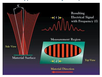
LaserSpeed uses dual-beam laser interferometer technology to measure product velocity (speed), which is integrated over time to measure length.
