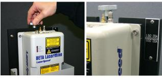
The LaserSpeed gauge is mounted to a heavy-duty sliding rail. A rotating knob enables you to adjust the gauge height, while the position indicator lets you precisely set the measurement distance for the specific product size.
